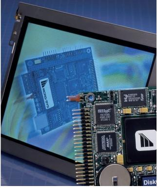
This embedded PC board has a 486-class cpu, VGA CRT and flat-panel LCD interfaces, RS-232 and RS-422/RS-485 serial ports, a printer port, digital I/O, a solid-state disk, and a PC/104 expansion bus.
