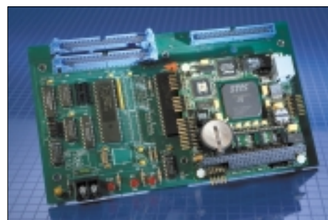
Figure 3 Example of a proprietary OEM controller board with a plug-in PC/104 module.
