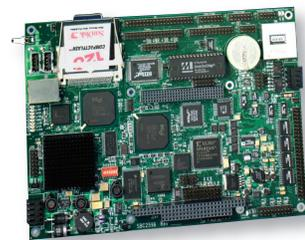
**Figure 1** A single board, such as this Micro/sys SBC2596, has three kinds of Linux drivers available: OS-supplied drivers for the serial and parallel ports, compact flash, USB and Ethernet. There are manufacturer-supplied drivers for A/D and D/A I/O and digital I/O. Finally, there is direct hardware access to the global positioning system.
