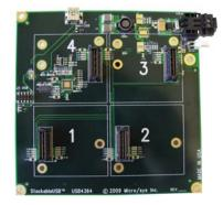
The CRR-NANO and the HUB-NANO provide a bridge from off-the-shelf Nano-ITX single board computers to the increasingly popular ¼-size StackableUSB I/O devices. Removina the burden of assessing compatibility from the OEM, the CRR-NANO and HUB-NANO securely mount top or bottom to any Nano-ITX form factor to provide access to multiple StackableUSB I/O modules. OEMs simply plug on their Nano-
