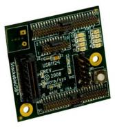
The USB1124 is a moderate-performance USB Client microcontroller board designed for low-power projects. Well-suited for applications confined to small, tight spaces, the 16 MIPS performance typically requires only 40mA power - figure small enough for battery-powered applications.
