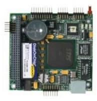
Netsock/435 provides a turnkey, network-oriented platform on which to build embedded systems. Based on the Micro/sys SBC1491 embedded PC and its built-in 10BASE-T Ethernet port, Netsock/435 is a powerful 486/586 computer that offers high performance, and that can significantly reduce development time.
