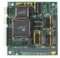
The MPC302 Dual Serial and Printer Interface adds two PC compatible COM ports and one parallel printer port to any PC/104 system. Complete control over I/O port addressing and interrupt IRQ selection is provided through settable jumpers. This allows standard and non-standard configurations to allow maximum flexibility in configuring PC/104 systems.
