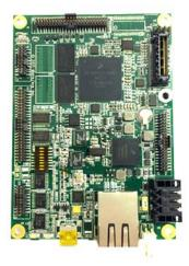
The SBC5651 is ideal for applications requiring small, low-power SBCs typical in medical, data collection, and test and measurement systems. With Freescale's i.MX515 ARM Cortex-A8 multimedia processor at its core, the SBC5651 effortlessly interfaces to a CSI CMOS camera module to offer functions such as OCR, bar code scanning, edge detection, and real time video or video capture. Users can control the speed and power consumption by adjusting processor speeds up to 800 MHz.
