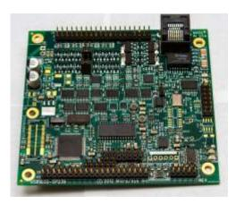
Ideal for data collection and data transmission, the USB3032 combines web hosting, networking, and industrial control. Multiple onbard protocols, including 10/100 Ethernet, CAN, RS232, RS485, USB, I<sup>2</sup>C, and SPI makes protocol conversion a snap. Microchip's PIC32 gives 125 DMIPS performance using under 100mA of power so the USB3202 is battery friendly with the 6-36V DC/DC option installed.
